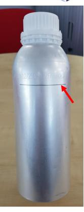
In the close up to the left, you can see that the 1 litre line sits just below the engraved manufacturers writing on the rear of the can, for reference it is around 8mm below this writing. We would suggest that it would be good practice to ensure that the can is filled to the level of the writing, so that it can be certain that the required 1 litre is present.
